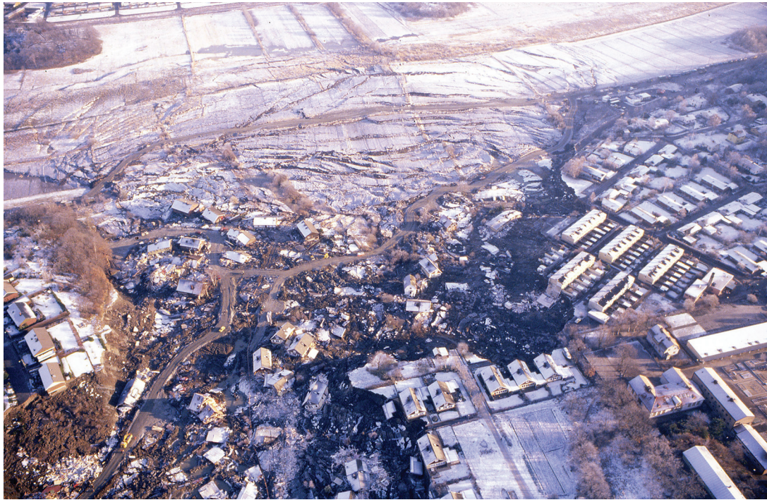
Fig. 14. Aerial photograph of the Tuve slide with East in the top. The slide started in the middle of the photo and moved beyond the Kville creek (top) © Gothenburg Museum of Natural History, reprinted with permission). [Color online.]
